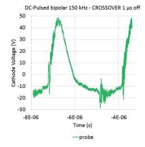
If the sputter target switches to a positive voltage, as the electrons are diverted to the anode, there is a strong positive ion bombardment of the film. This enhances hardness and density.
