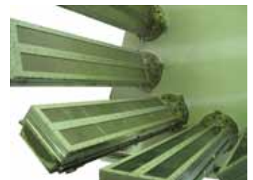
Web coating configuration involving multiple rectangular magnetrons
