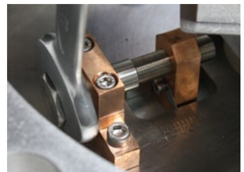
Figure 2: Adjusting the location of the magnetic pack can be easily carried out, and without dismounting the magnetron
