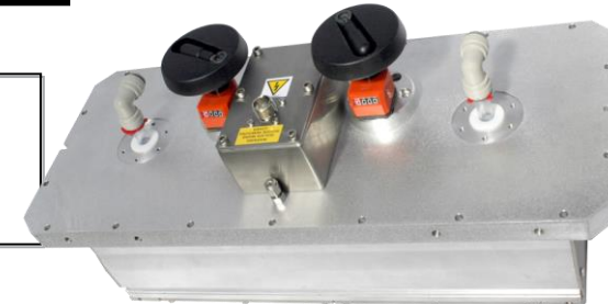
VT100300 fully balanced position B_z=0 @ 80mm
