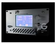
The built-in software can drive external mass flow controller to mantain the source voltage at a preset value. The features of the iM300 and iM3000 ensure that the setup, operation and regulation of the plasma source is straightforward.
