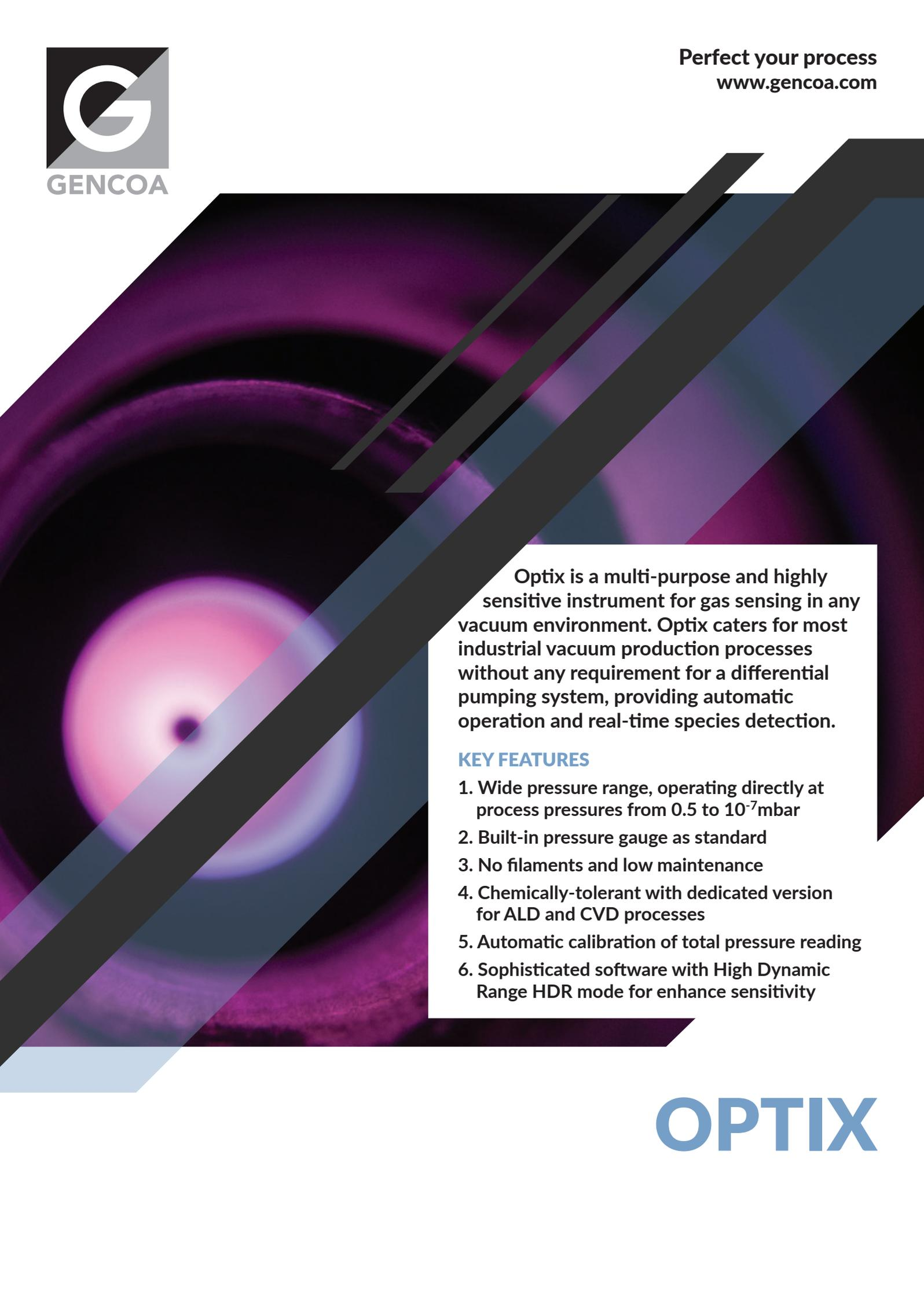
Optix is a multi-purpose and highly sensitive instrument for gas sensing in any vacuum environment. Optix caters for most industrial vacuum production processes without any requirement for a differential pumping system, providing automatic operation and real-time species detection.
