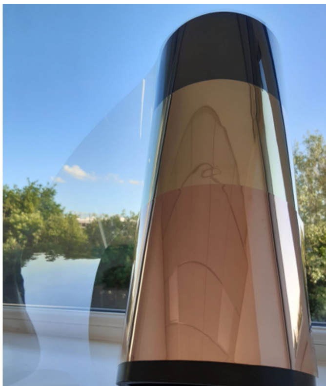
Fig. 14 – Three different forms of copper based biocidal vacuum coatings on PET film: from the top, transparent, gold effect and pure copper.
