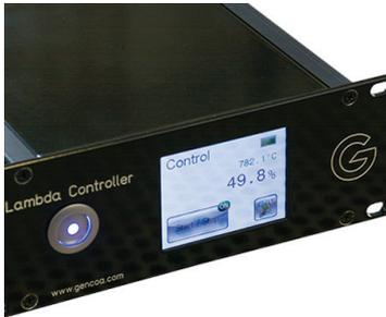
The sensing method uses a zirconium oxide ceramic (zirconia - lambda sensor) and is based on a solid-state electrochemical fuel cell called the Nernst cell. Its two electrodes provide an output voltage corresponding to the quantity of gas in the vacuum relative to that in atmosphere.
